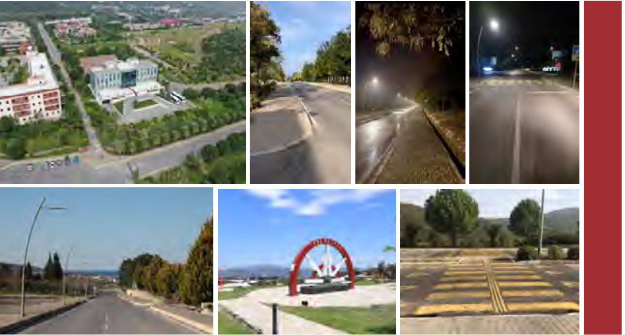
Figure 10: At IZTECH, all sidewalks are lightened and separated from the roads by elevation. The sidewalks are designed as accessible for physically disabled persons. All crosswalks are marked with pavement markings and traffic signs. The elevated crosswalks are used as speed ramps for speed limit enforcement especially where the pedestrian traffic is high.
